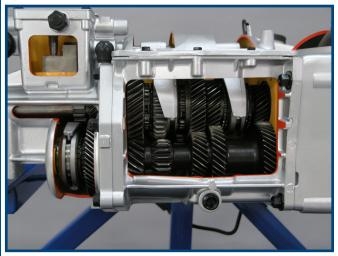
This trainer presents a Rear Wheel Manual Transmission that allows for demonstration of shifting and clutch operation.
