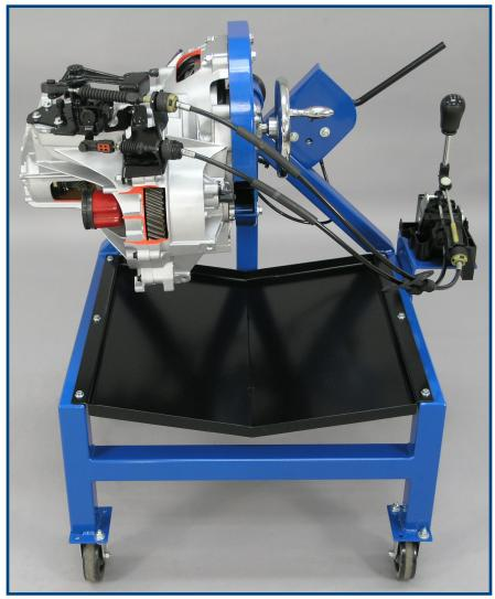
This trainer presents a Front Wheel Drive Manual Transaxle that allows for demonstration of shifting and clutch operation.
