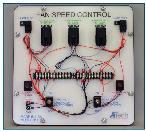
This ATech Trainer presents the hands-on construction, study and live operation of a modern Fan Speed Control System as found on late-model General Motors vehicles. Students follow printed schematics to wire up either a single-speed single fan system or a two-speed two fan system. The trainer circuits use the same wire colors as the manufacturer's wiring diagram. Incandescent bulbs are substituted in place of the actual cooling fan motors for safety purposes.
