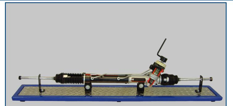
The Power Rack and Pinion Cutaway (model 507) trainer is a cutaway of an actual power rack and pinion that shows internal components, allowing demonstration of internal components.
