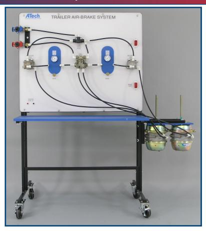
The Trailer Air Brake (model 6420) trainer presents the "real world" operation and study of a Trailer Air Brake System. The trainer is capable of duplicating actual on-vehicle problems. The program provides courseware for use by students and instructors.
