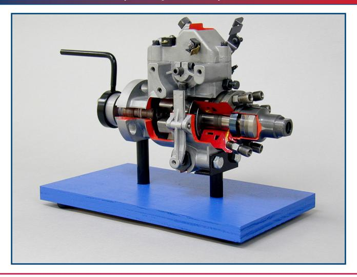
The Diesel Rotary Injection Pump Cutaway (model 6681) provides hands-on experience. The cutaway shows the internal components of an electronic fuel control and cold advance injection pump.
