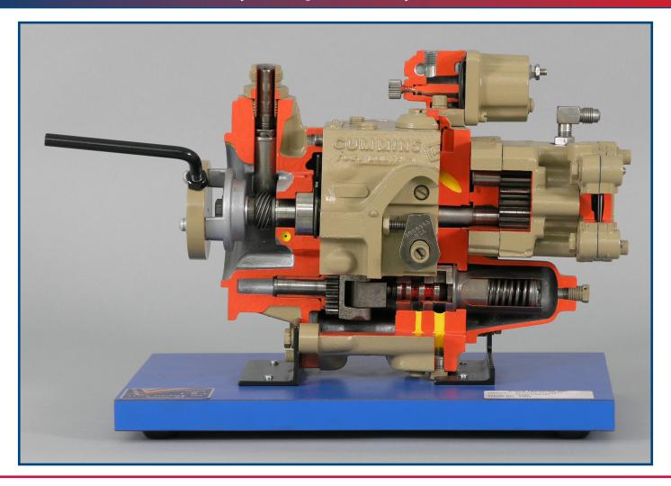
The Diesel Rotary Pump Cutaway (model 6682) provides hands-on experience. The cutaway shows the internal components of an electronic fuel control and cold advance injection pump.
