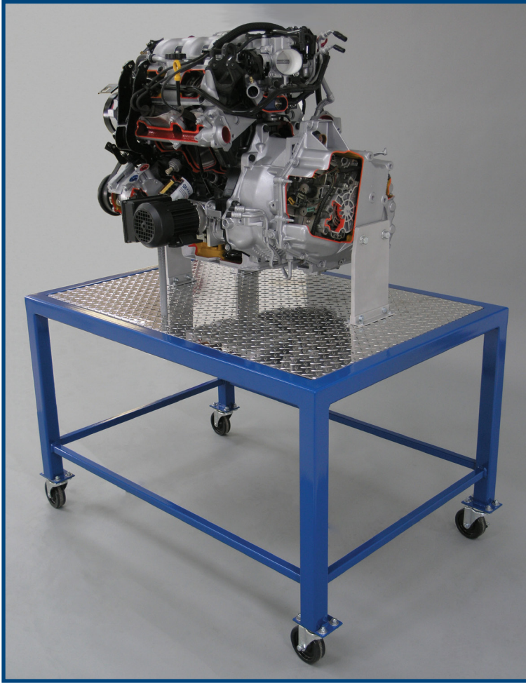
GM Six-Cylinder Cutaway SIDE VIEW (model 680)
