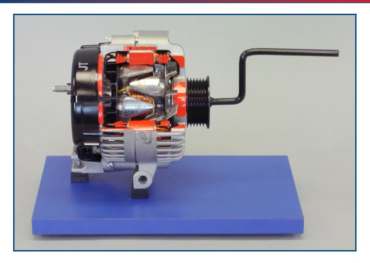
The Alternator Cutaway (model 814) is a cutaway of an actual alternator that shows internal components, to demonstrate alternator operation.
