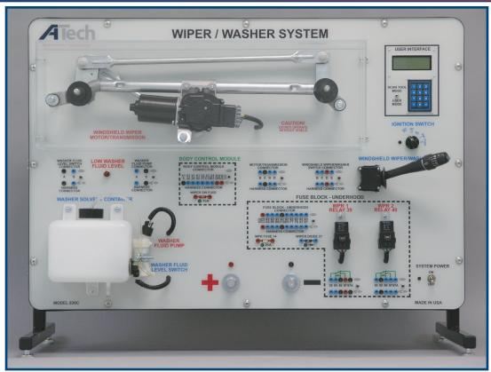
The ATech Wiper/Washer System Trainer (model 830C) is part of an electrical system program which presents the live operation and study of wiper/washer systems. This trainer allows for instuctor demonstration, student hands-on reinforcement and troubleshooting practice. Powered by a 12VDC automotive battery or a 12VDC/23A power supply (not included).
