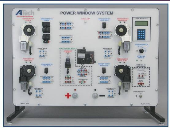
The ATech Power Windows System Trainer (model 840C) is designed to teach computer and network controlled automotive power window operation. This trainer allows for instuctor demonstration, student hands-on reinforcement and troubleshooting practice. Powered by a 12VDC automotive battery or a 12VDC/23A power supply (not included). The Power Windows System is based on a CAN platform vehicle.
