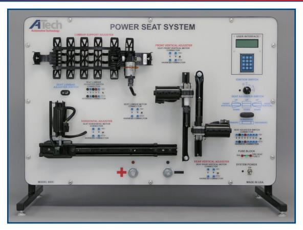
The ATech Power Seat Trainer (model 860C) is part of an electrical system program which presents the live operation and study of power seat systems. This trainer allows for instructor demonstration, student hands-on reinforcement and troubleshooting practice. Powered by a 12VDC automotive battery or 12VDC/30A power supply (not included). The Power Seat System is based on a CAN platform vehicle.
