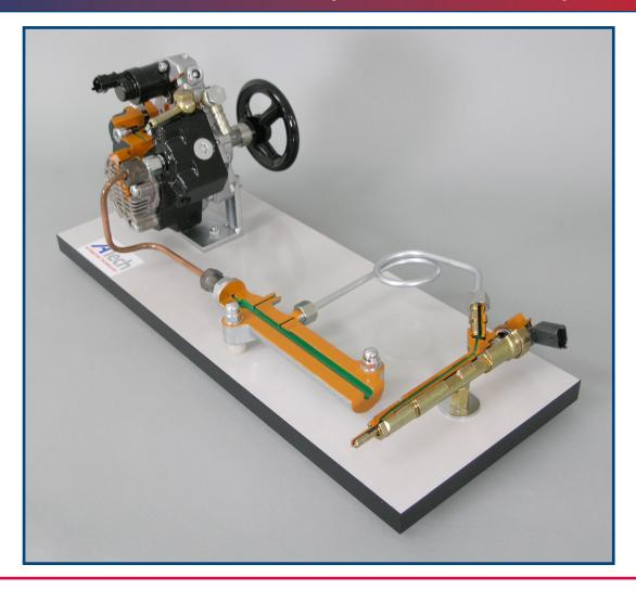
This model shows an accurate cross-section of the high pressure (1300 bar) fuel system known as common rail. This circuit consists of a radial piston pressure pump, one delivery manifold, and an electro injector, all connected via high pressure hoses.
