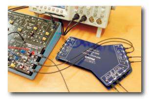
The ETT-101-31 FIBER OPTIC COUPLERS and WDM FILTERS Experiment expansion board includes four independent functional blocks. When added to the ETT-101 and ETT-101-31 it will allow a complete bi-directional and WDM fiber optic links to be implemented.
