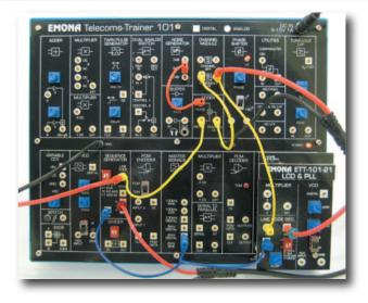
Patching a line-code encoding & decoding experiment with signals passing through a noisy bandlimited channel uses 6 of the ETT-101's functional blocks:
