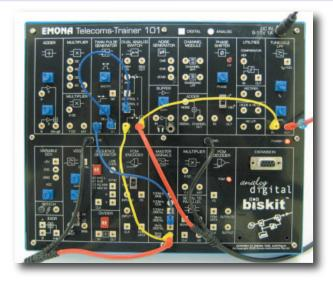
Patching a sampling & reconstruction experiment uses 4 of the ETT-101's functional blocks: MASTER SIGNALS, TWIN PULSE GENERATOR, DUAL ANALOG SWITCH and TUNEABLE LPF
