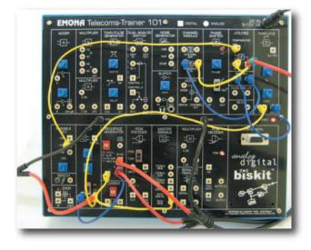
Patching an FSK modulation and demodulation experiment uses 7 of the ETT-101's functional blocks: VCO, SEQUENCE GENERATOR, MASTER SIGNALS, BANDPASS FILTER, UTILITIES, VARIABLE DC V and TUNEABLE LPF.
