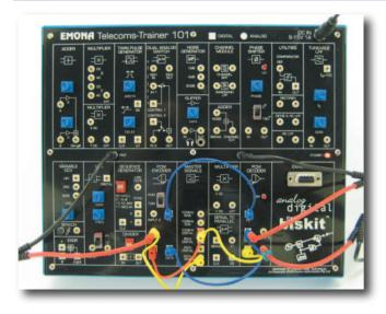
Patching a PCM encoding & decoding experiment uses 3 of the ETT-101's functional blocks: MASTER SIGNALS, PCM ENCODER and PCM DECODER.
